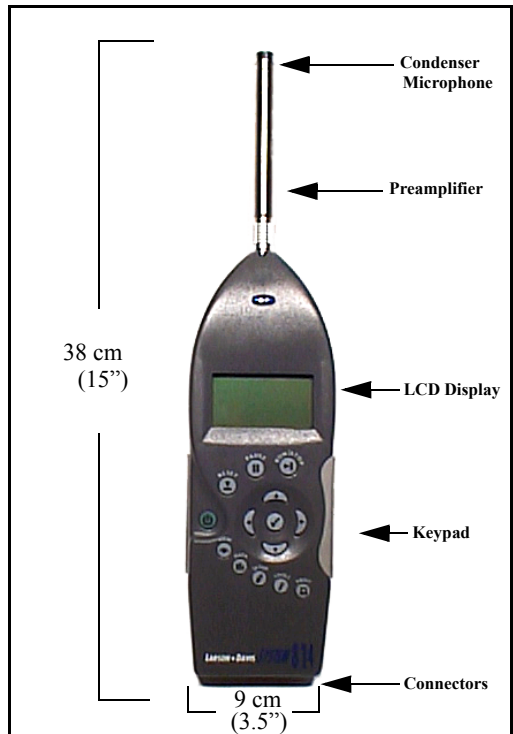
Figure 1-1 The System 824 is a convenient hand-held sound level meter with a simple user interface.
