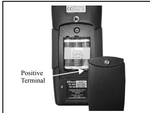
Figure 1-7 Battery compartment and cover with NiMH battery pack installed. (Note location of positive terminal.)
