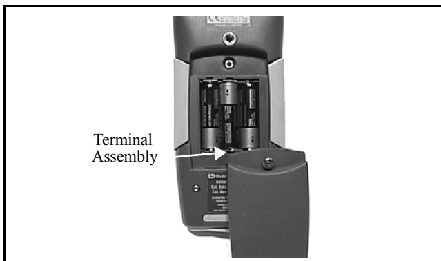
Figure 1-9 Battery cover and compartment with alkaline batteries and Terminal Assembly installed. (Note location of Terminal Assembly.)
