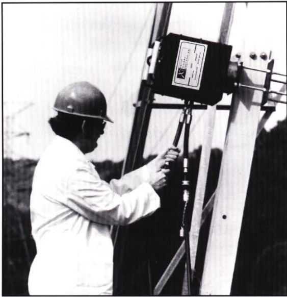
Xcite 1100-5 System used to test a utility tower
