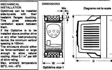
MECHANICAL DIMENSIONS Optidrive Optidrive Optidrive Optidrive Size 1 Size 2 Size 3 Size 4 Length 155mm 260mm 260mm 520mm (L) Width 80mm 100mm 171mm 340mm (W) Depth 130mm 175mm 175mm 220mm (Ď) Width to screw centre 9.5mm 4mm 4mm 4mm (Ws) Length to screw centre 25mm 25mm 50mm 25mm (Ls) Number of 2 x M4 2 x M4 4 x M4 4 x M8 fixing screws
