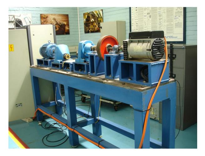
Length:2.6m (Maximum shaft length of 1.5m between the<br/>Electric motor and alternator)Width:0.5mHeight:1.06mCentre height:130mm (min)Mounting slots:none
