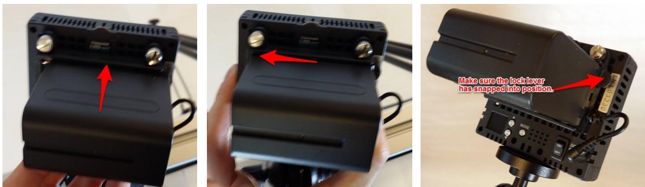
Figure 15: Attaching the battery to the LED unit.
