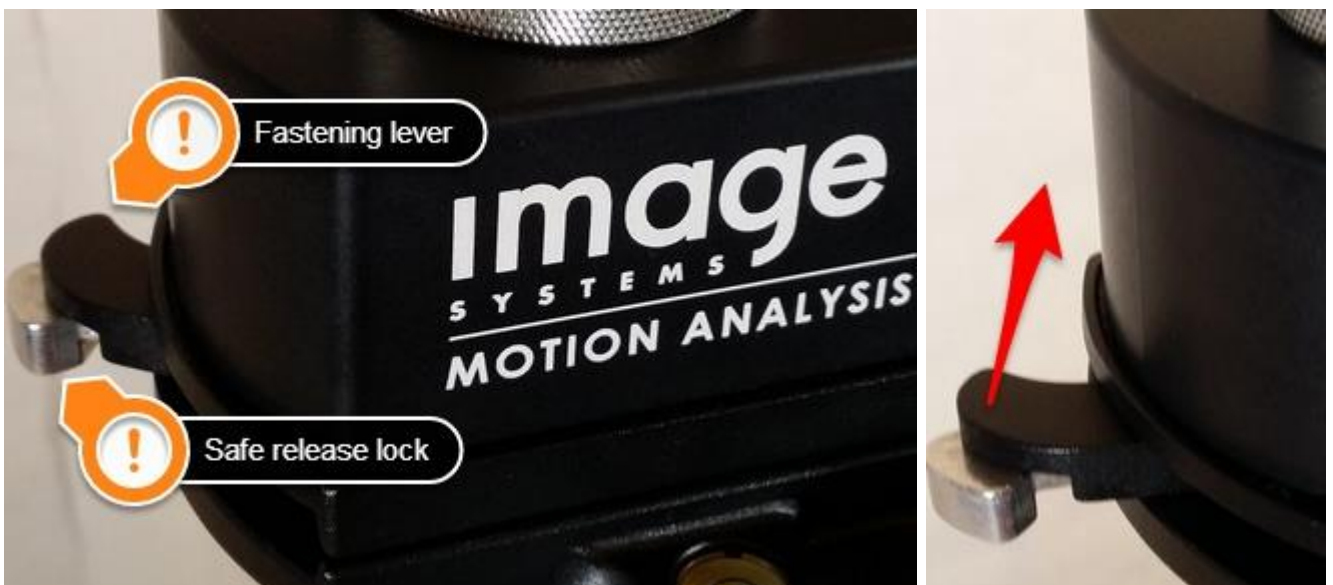
Figure 10: Tighten the lever holding the mount bar in place (left). The fastening and safe release lock on the lever (right).
