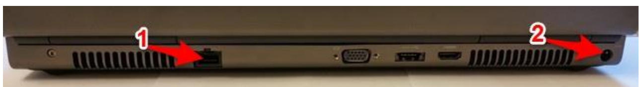
Figure 17: Laptop connectors. Ethernet connector (1) and power cord (2).
