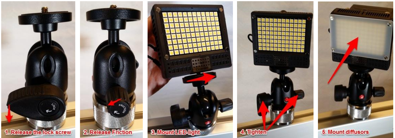
Figure 14: Mounting the LED lights.
