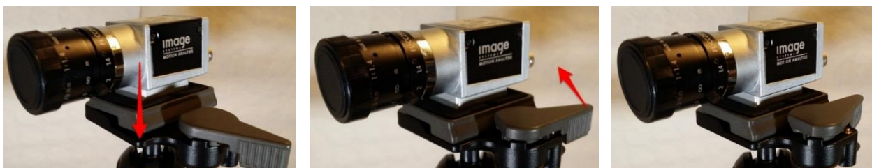
Figure 13: Mount the camera on the camera mount.
