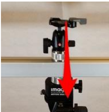
Figure 9: Snap the mount bar onto the tripod.
