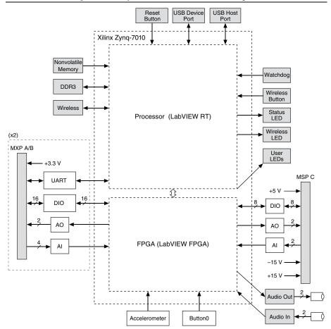
Figure 2. NI myRIO-1900 Hardware Block Diagram
