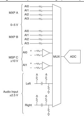
Figure 5. NI myRIO-1900 Analog Input Circuitry
