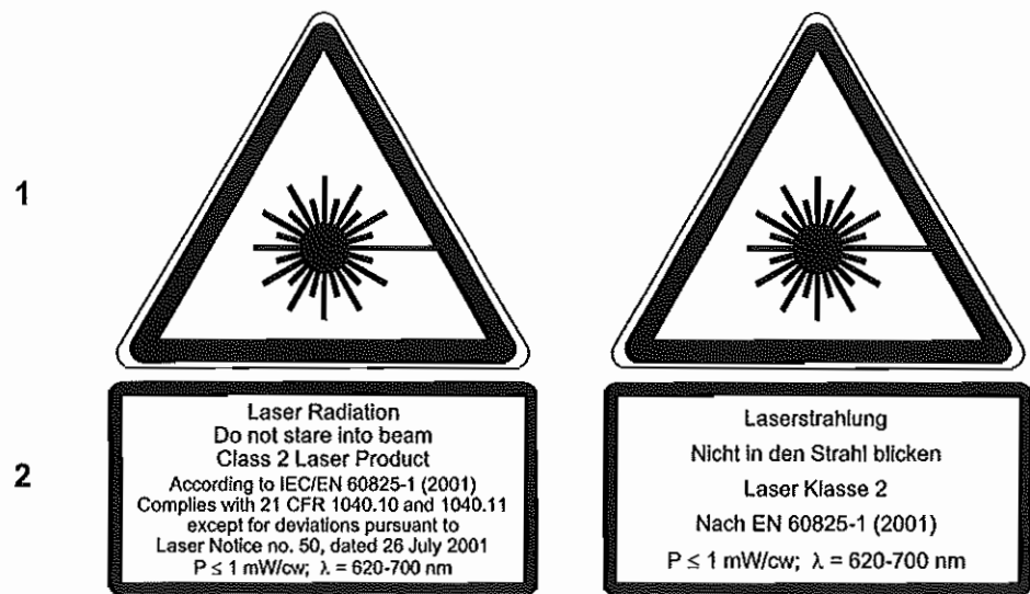
Figure A.1: laser warning labels for the scanning head with geometry scan unit
