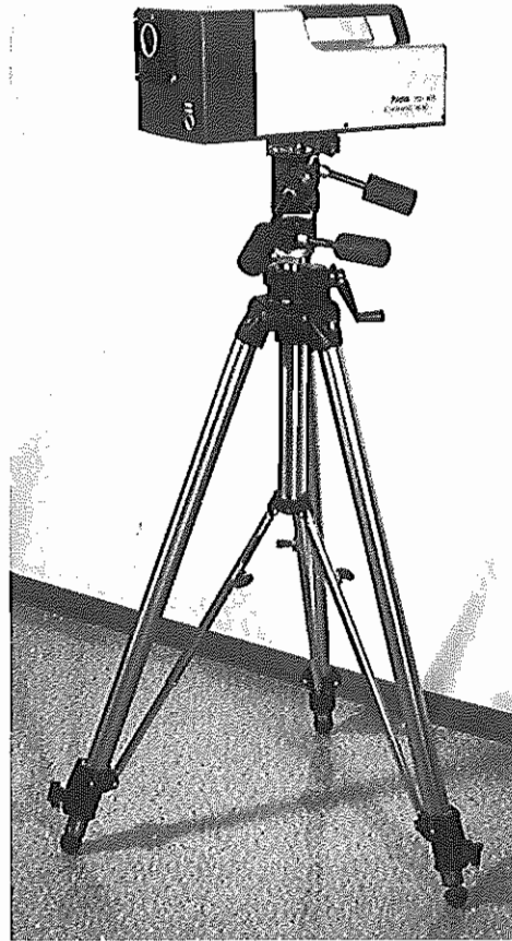
Figure 3.18: Scanning head mounted on the tripod with fluid stage
