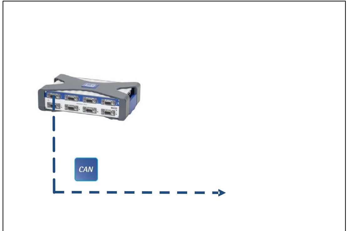
Fig.5.9: Output to CAN bus (MX840A, connection 1)
