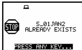
Displays after SAVE operation when the file with the selected name already exists in the instrument's memory (with the message if REPLACE is not active)
