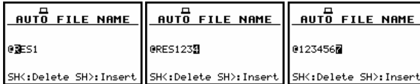
Displays after entering FILE NAME edition mode for the files saved with AUTO SAVE option active (after pressing <ENTER> push-button in SAVE OPTIONS window, AUTO SAVE switched on)
