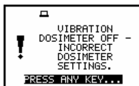
Display after starting measurements when user selected incorrect filters for HAV/WBV DOSE calculations
