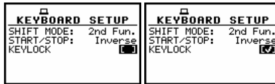
KEYBOARD SETUP window with the activation of KEYLOCK option
