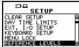
SETUP list with REFERENCE LEVELS text highlighted (displayed inversely)
