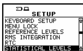
SETUP list with STATISTICAL LEVELS text highlighted (displayed inversely)
