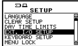
SETUP list in sound measurements with EXT. I/O SETUP text highlighted (displayed inversely)
