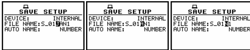
Displays in FILE NAME edition after pressing <Shift> and << push-buttons
