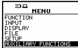
Main list with AUXILIARY FUNCTIONS text highlighted (displayed inversely)
