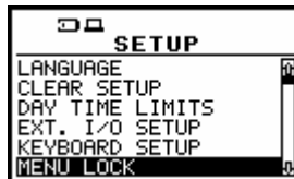
SETUP list with MENU LOCK text highlighted (displayed inversely)
