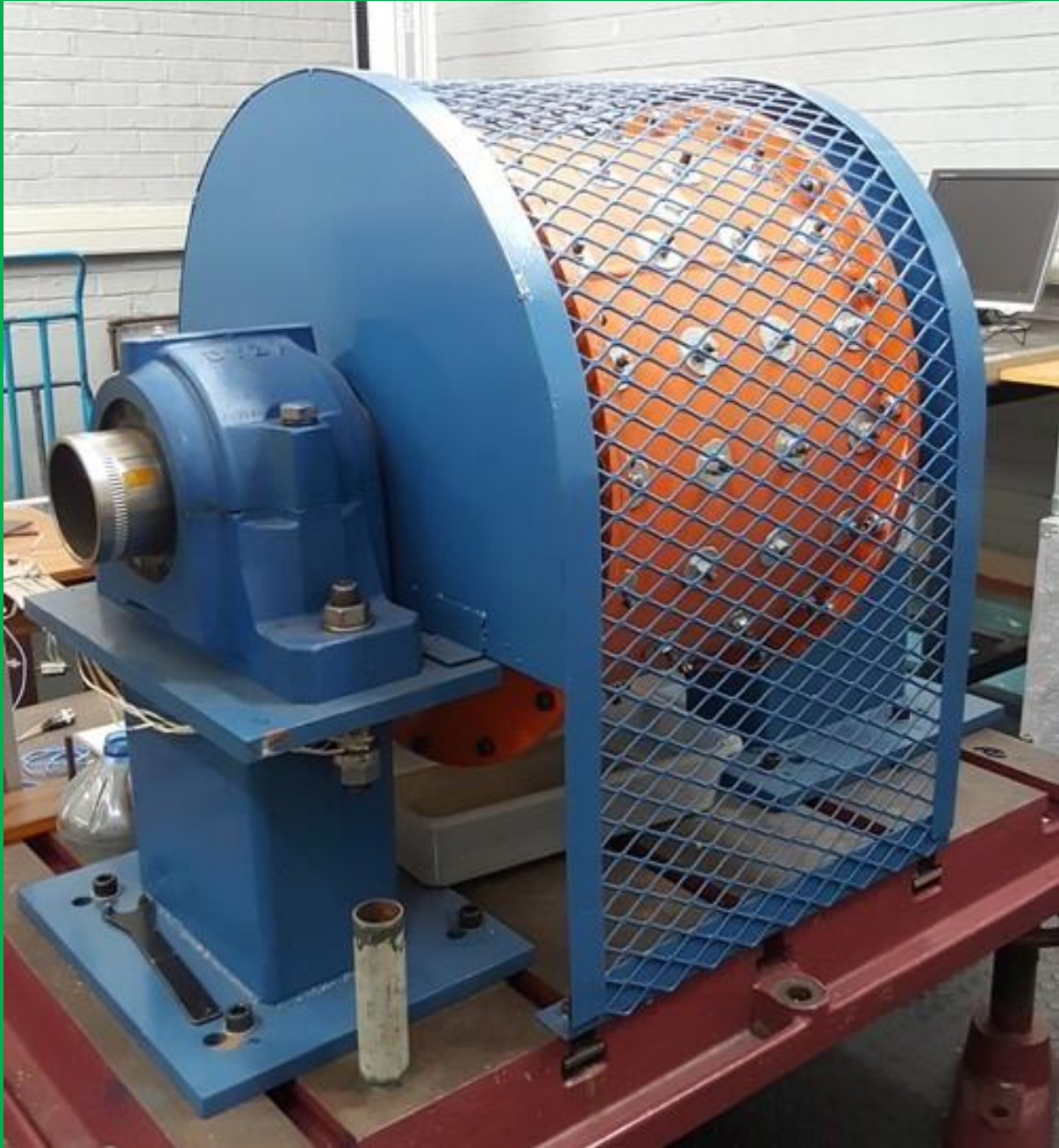
New SAG MILL experimental test bench Ready for use
