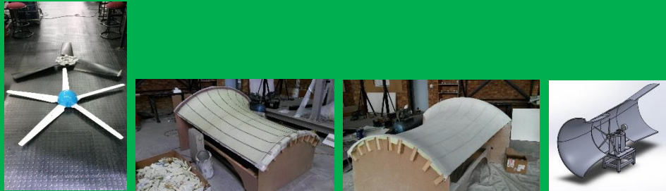
Images showing the Turbine and Fan blades and construction of the tunnel intake
