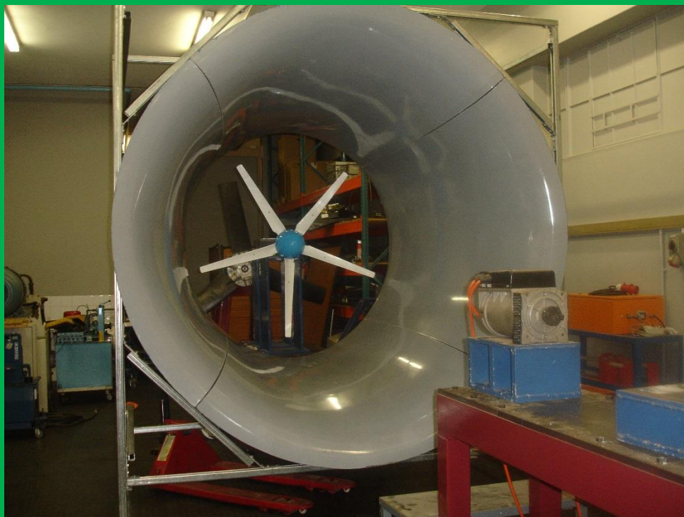
The tunnel intake and turbine rotor in position
