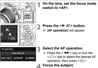
Aim the AF point over the subject and press the shutter button halfway. The camera will then autofocus in the selected AF operation.
