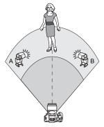
Divide the slave units into groups A and B and change the flash ratio to obtain the desired lighting effect. Refer to your Speedlite's instruction manual to set one slave unit's slave ID to A (Group A) and the other slave unit's ID to B (Group B), and position them as shown in the illustration.
