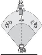
This is convenient when you need a large flash output. All the slave units will fire at the same output and be controlled to obtain a standard exposure. No matter what the slave ID is (A, B, or C), all the slave units will fire as one group.
