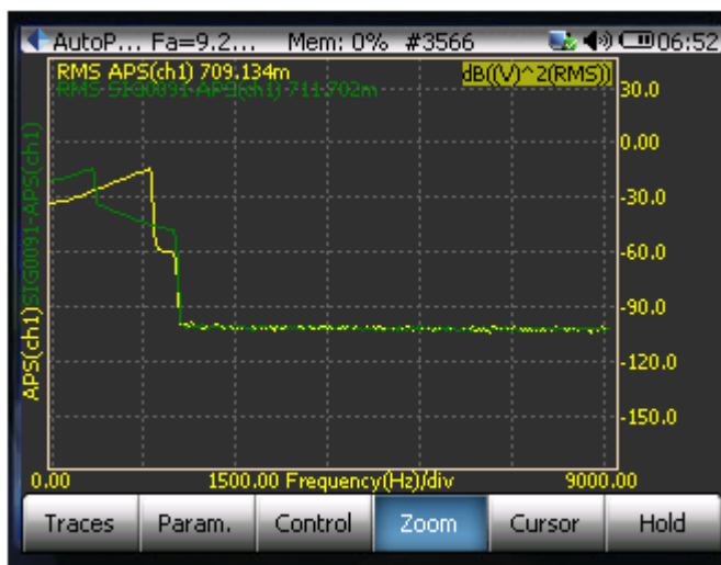
■ Figure 78. Live signal overlaid with recalled signal.
