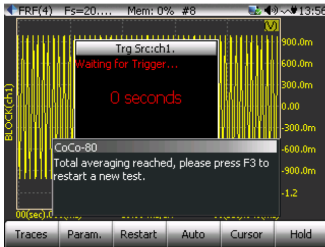
■ Figure 129. When averaging is complete you can restart a new test with the Run Button.
