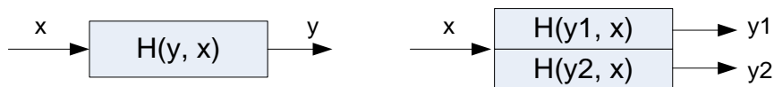
■ Figure 1 Left: a UUT with one response; Right: a UUT with two responses.
