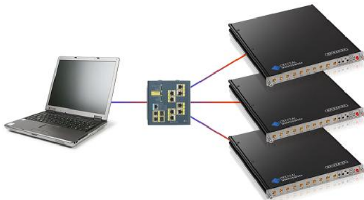
■ Figure 27: Computer private LAN with router and multiple Spider modules
