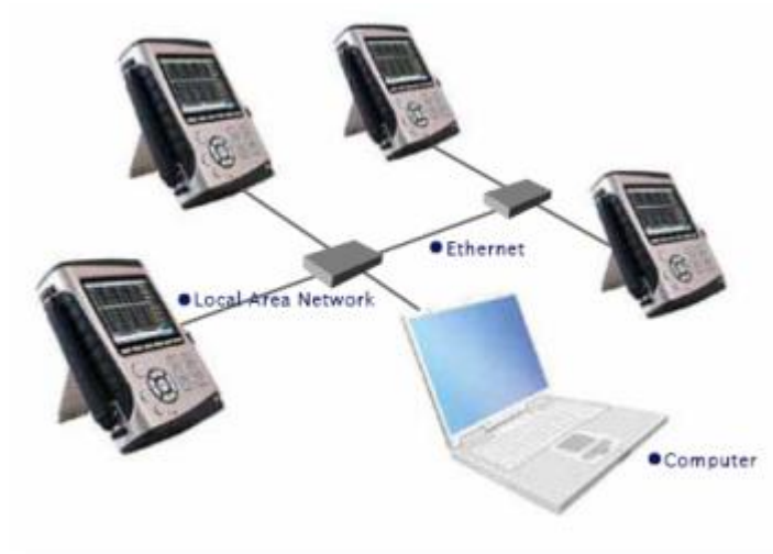
■ Figure 40. Remote operation for multiple CoCo units with automated testing.
