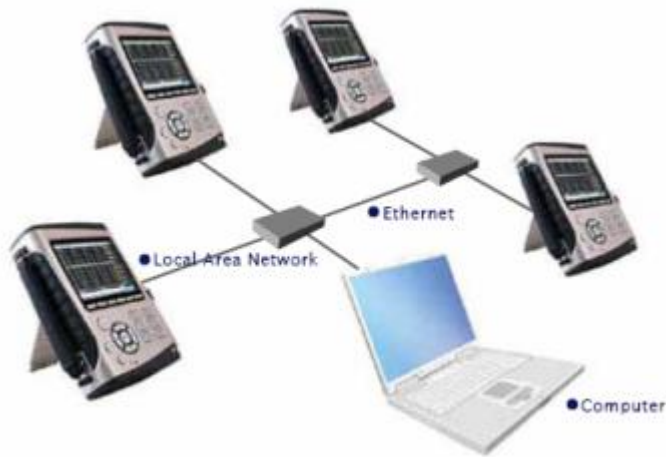
■ Figure 117. Remote operation for multiple CoCo units with automated testing.
