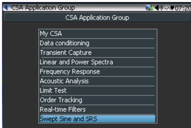
■ Figure 109. SRS CSAs are saved in the Swept Sine and SRS application group.
